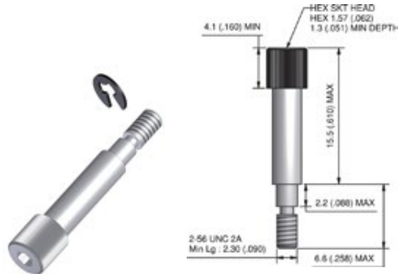
KIT PART NUMBER: MDAHM503 According to M83513/05-03 Hardware code: N
