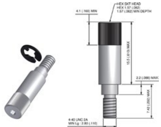
KIT PART NUMBER: MDAHM513 According to M83513/05-13 Hardware code: N
