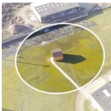
▲ FIGURE 1: Location of magnetic test facility (30m away from possible interference)
