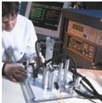
▲ AUTOMATIC CONTINUITY & INSULATION RESISTANCE TEST
